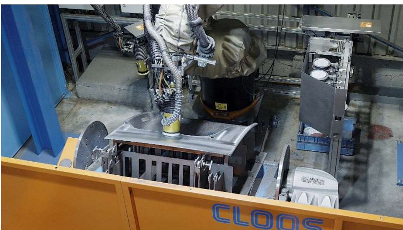
Photo 4: The robot also takes care of the fine grinding.
