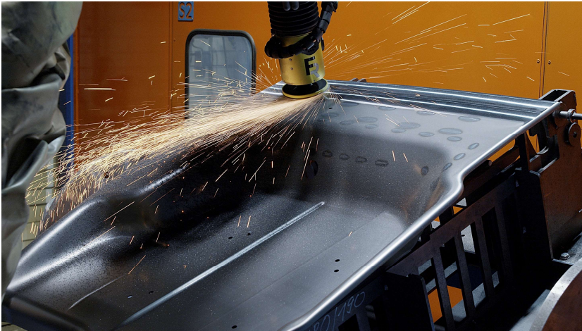
Photo 2: This is followed by the automatic grinding process.
