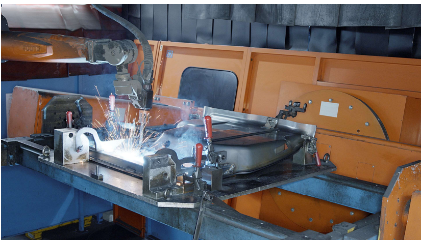
Photo 1: First, CLOOS robots weld the components.
